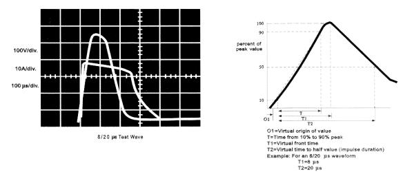
It must note one thing that the rated energy and the energy absorbed in a Varistor may not be identical. It has a situation that a ZnO varistor with better clamping voltage will absorb less energy. It is very important to emphasize that poorer ZnO varistor will absorb higher energy in the ZnO varistor itself and the better ZnO varistor which performs a lower clamping voltage will absorb less energy, yet actually provides a better over-voltage protection.
